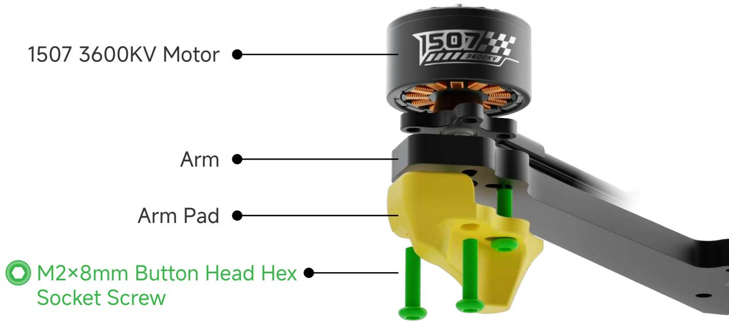
Note: Motors and motor wires are not included in the package
